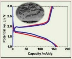
Galvanostatic cycling behavior for TiO2 nanotube electrodes at a rate of C/10 vs. Li
