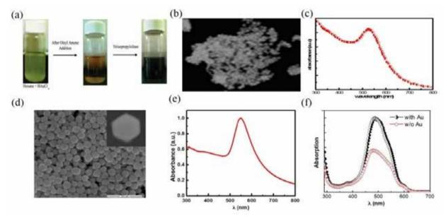
Figure 2: (a) Synthesis of Au nanosphere (b) Au nanosheres of size ~ 10 nm (c) UV-Vis absorption spectra (d) Truncated octahedral Au nanoparticles of size ~ 65 nm (e) UV-Vis absorption spectra of Au NPs (f) UV-Vis absorption spectra of P3HT: PCBM with and without Au NPs.
